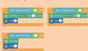
In order to change speed in real time, VinciBot needs to constantly detect the distance to the obstacle. To do this, not only does "forever" need to be used, but the "nested if else" statement is also required to program.
